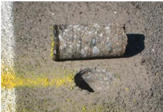
**Fig 1** Core sample showing well bonded sprayed seal on bitumen stabilised base
