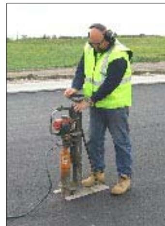
Figure 1: Coring machine with guide frame
